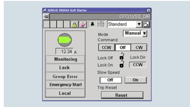
Faceplate of the motor block
